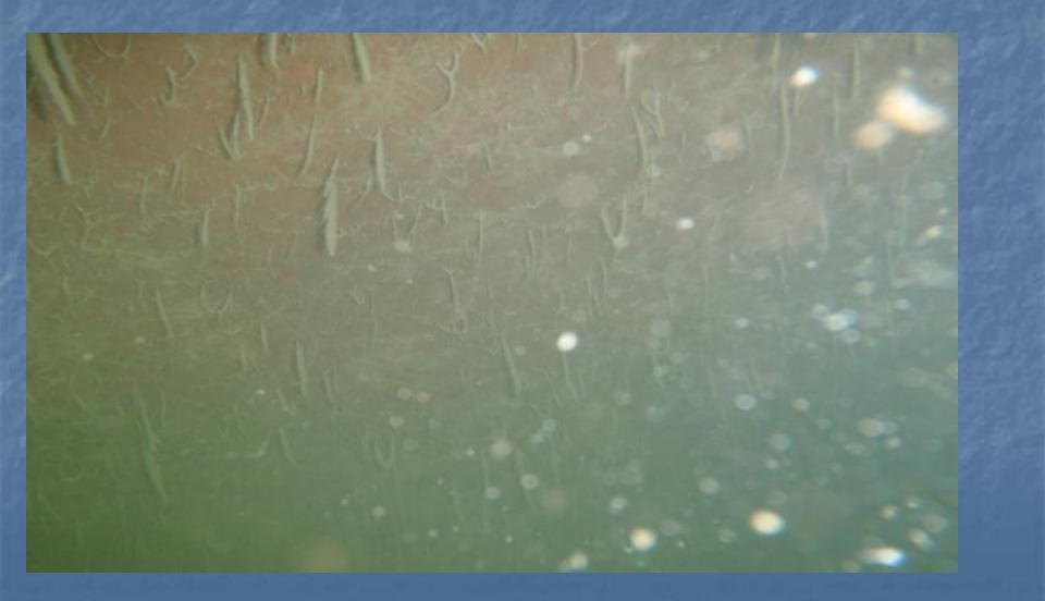
Heavy fouling Silt Layer on hull Paints Pigment may be difficult to determine Moderate to Heavy 3D growth Present on Boat and Running Gear Cleaning Type 4 growth will result in Paint Loss
