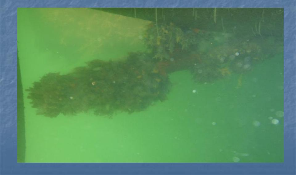
Heavy Silt Fouling 100% Vessel
